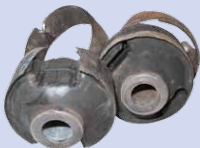
Metal outer ring separated from rubber bushing
