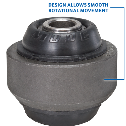
SEALED MOOG POLYURETHANE BOOT KEEPS CONTAMINANTS OUT
