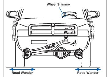
**NOTE:** Determine the condition of the track bar using the OE inspection procedure. Track bar pivot assemblies exhibiting more than .080" of movement should be replaced. Some technicians have reported wheel wander and road shimmy with pivot assembly deflection below the .080" OE specification.
