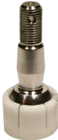
Non-serviceable plastic design has failed due to intrusion and wear.
