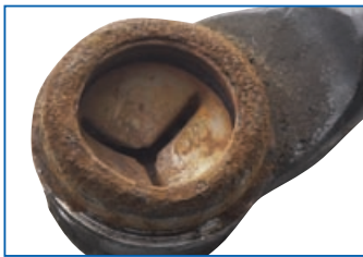
Non-serviceable plastic design has failed due to intrusion and wear.
