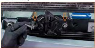
06. Remove the two bolts that secure the cooler to the radiator support and lower the cooler. (2x 10mm bolts)
