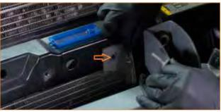
07. Remove the bolt that secures the horn assembly to the radiator support. Then lay the horn assembly over the intercooler. (1x 10mm bolt)
