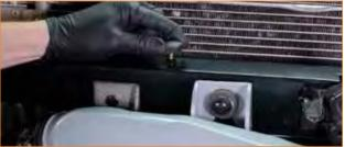
22. Gently close the hood and press it down to engage the latch. If the latch does not engage, the bump stops are too high or the latch is too low. If the latch engages, but the hood is too low, the bump stops need to be raised. Adjust the height of the latch and the bump stops until latches properly and the hood is flush with the fenders. This may take a few tries to get it just right.
