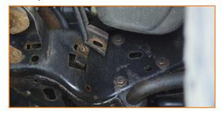
3. Remove the bolts and brackets that secure the front bumper. (6x 18mm bolts)
