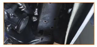
2. Remove the bolts where the frame ends meet the bumper. (2x 18mm bolts)
