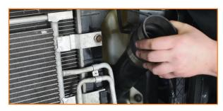
Mark the transmission cooler hoses. It's recommended that the mark be five inches back from the hump. Once done, cut the hoses on your mark.
