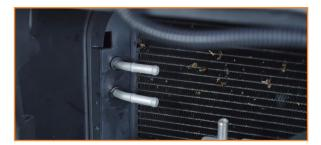
16. Connect the cooler lines to the adapters. Transfer the two safety caps to the new lines.
