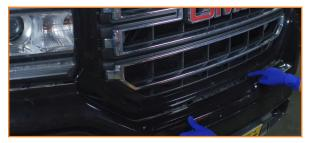
Take out the bolts that secure the grille. This includes all hardware along the bottom and top. (8x 10mm bolts)
