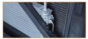
Secure the transmission cooler with your mounting hardware. If the cooler is crooked and needs to be adjusted, loosen the button head bolts on the backside of the cooler brackets to adjust its position. (2x brackets, 4x Allen bolts)
