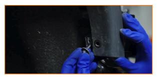
Disengage the bumper cap at the sides and along the bottom of the grille. There are a number of tabs just under the grille that will release this piece. Remove the loose bumper cap. (2x 7mm bolts)
