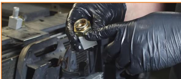
10. Attach the adapters to the transmission cooler line. You will hear an audible click when the fittings are set. Then slide the clip covers over the connection. (2x ring clips)
