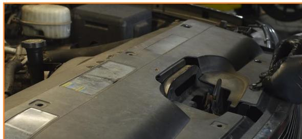
2. Pull back the edges on both sides of the grille. This will release the tabs holding the grille. Once the tabs are free, remove the grille.
