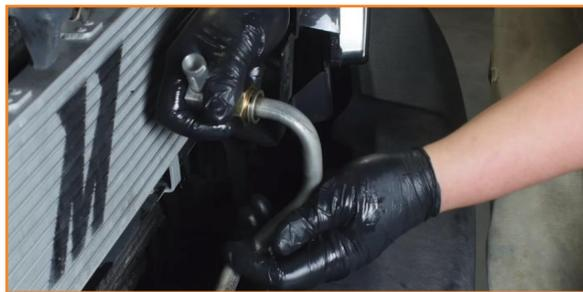
11. Install the provided hoses to the transmission cooler ports. Then attach the cooler lines to the hoses you just installed. (4x worm gear clamps)
