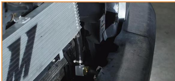
12. Reinstall the front grille. Engage the taps at the sides.
