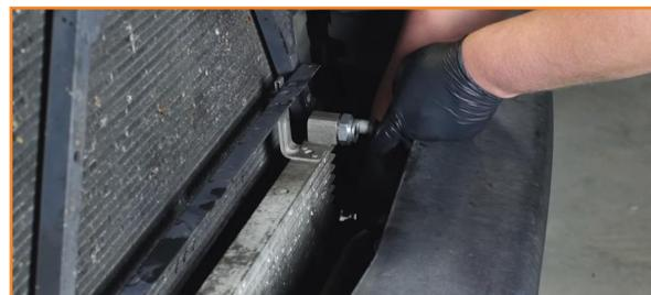
4. Disconnect the cooler lines from the transmission cooler. Use a pick tool to slip off the clips that secure these lines. (2x ring clips)
