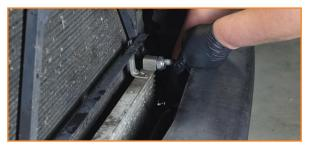
4. Disconnect the cooler lines from the transmission cooler. Use a pick tool to slip off the clips that secure these lines. (2x ring clips)
