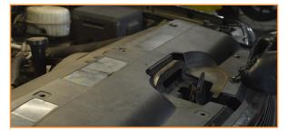
2. Pull back the edges on both sides of the grille. This will release the tabs holding the grille. Once the tabs are free, remove the grille.
