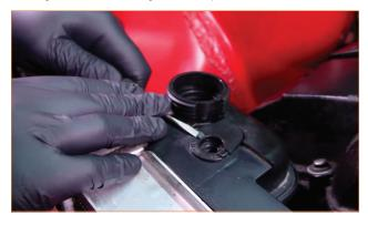
**04.** Loosen the worm-gear clamp connecting the expansion tank and the overflow hose. To locate the clamp, tilt the expansion tank toward the motor, and look through the hole from which the bleeder screw seal was removed. Pull the overflow hose off the expansion tank. (1x worm-gear clamp)
