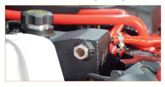
12. Remove the filler plug from the expansion tank, and fill the lower section of the tank until the coolant reaches about halfway up the sight tube. Then reinstall the filler plug.
