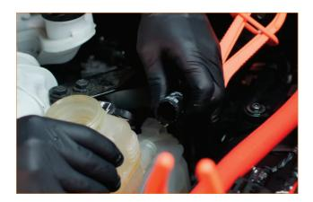
06. Remove the mounting grommet from the stock tank and transfer it to the Mishimoto tank. (1x rubber grommet)
