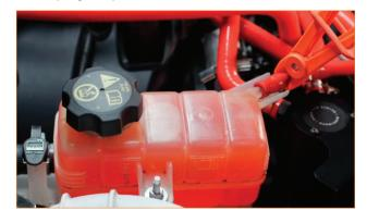
02. Remove the nut that secures the expansion tank to the vehicle. (1x 10mm nut)
