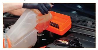
05. Once you have drained the coolant below the port at the bottom of the expansion tank, pinch off the coolant hose, compress the clamp that secures it, and separate the hose from the tank. Now remove the tank from the vehicle and drain the remaining coolant.
