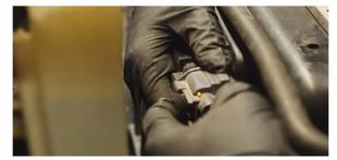
Compress the clamp that secures a small hole to the port on the overflow tank, and slide the clamp down the hose. Then pull the hose off the port. (1x spring clip)
