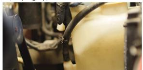
13. Remove the overflow tank. Be careful not to spill any coolant during this step.
