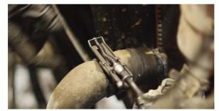
Disconnect the fan shroud's electrical harness. Depress the grey tab at the center to release the connection. Then pull the clip that holds the wiring out of the bracket on the fan shroud. (1x tree-clip)
