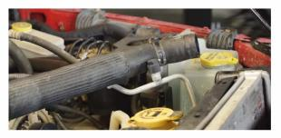
10. Compress the clamp on the lower radiator hose and slide it down the hose. Then pull the hose off the radiator port. (1x spring clamp)
