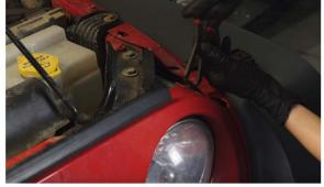
3. Disconnect the electrical harness located on the bottom of each side of the grille. To disconnect this harness, lift the red tab and then depress the black tab at the center.
