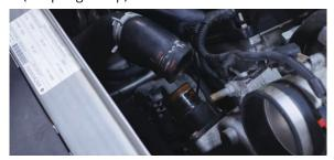
20. Compress the clamp on the upper radiator hose and move it down the hose. Then separate the hose from the radiator. (1x spring clamp)
