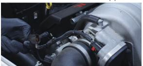
16. Loosen the clamps on each end of the intake pipe where it connects to the throttle body and filter. Our loaner vehicle had an aftermarket intake installed. Expect that yours will look different compared to the one shown here. (2x worm gear clamps)
