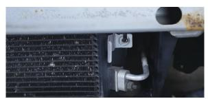
14. Remove the bolts that secure the AC condenser to the radiator, which includes the two radiator stays located on the top brackets. (4x 10mm bolts)
