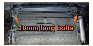
**18.** Install the Mishimoto radiator in the reverse order of removal using the provided hardware. See above images for hardware locations.
