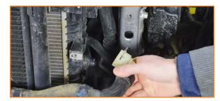
17. Remove the two bolts that secure the AC condenser. (2x 10mm bolts)
