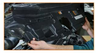
3. Remove the bolts at the top of the grille. Pull the grille off the front of the truck. Note the orange tabs on the inside for when you must reinstall the grille. (8x 10mm bolts)
