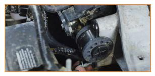
12. Separate the airbag sensor from the upper support bar. Simply remove the screw. DO NOT disconnect the harness. (1x 8mm bolts)
