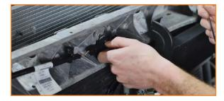
13. Release the petcock to drain the coolant from your primary and secondary radiators. Have a bucket ready to catch the released coolant. Unscrew the filler cap to expedite the draining process.
