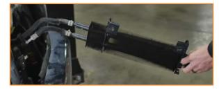
14. Release the power steering cooler and move it out of the way. (1x tree clip)
