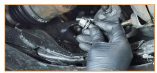
10. Angle the larger bracket in your kit up into the engine bay. Install the larger bracket to the steering rack using the same bolt from the previous step. Do not fully tighten the bolt yet. You will return to this later. (1x 14mm bolt)
