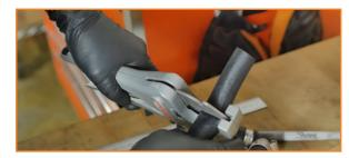
14. Combine the two shorter hoses using the 90° fitting to make your outlet hose.(2x worm gear clamps)
