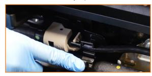
3. Remove two bolts behind the fuel line. (2x 10mm bolts)
