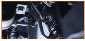
12. Compress the clamp on the lower radiator hose and slide the hose off the port.
