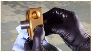
**30.** Orient the adapter so that the threaded ports on the sandwich plate face toward the front of the vehicle, and torque the center bolt to 30 ft-lb.
