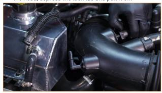
17. Remove the last hose from the intake pipe by sliding the lock tab down the slot and pulling it off the port.
