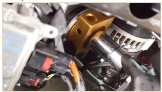
**31.** Install the two provided AN fittings to the sandwich plate and tighten them completely. (2x 1" AN fittings)
