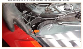
13. Pull outward on the bumper where it meets the fender to release it from the vehicle. Do this on both sides.
