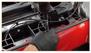
12. Remove the two small screws that secure the top of the bumper, located just inboard of the headlight assemblies, underneath the hood seal. (2x 5.5mm screws)
