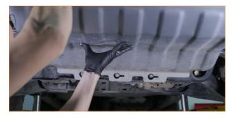
**03.** Remove the four tree clips that secure the air diversion panel to the underside of the fan shroud. (4x tree clips)
