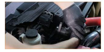
**08.** Remove the eight pop clips that secure the cover to the radiator support and fan shroud. Then remove the cover from the vehicle. (8x pop clips)
