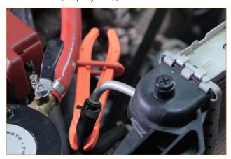
18. Now repeat this process on the lower transmission cooler line. (1x spring clamp)
