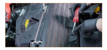
09. Separate the transmission cooler lines from the clips that secure them to the fan shroud.
