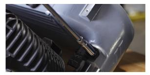
22. Slide the provided clip nuts onto the intercooler's lower brackets.
