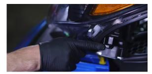
3. Remove the pop-clips that secure the undertray to the stabilizer bar. (2x pop-clips)
