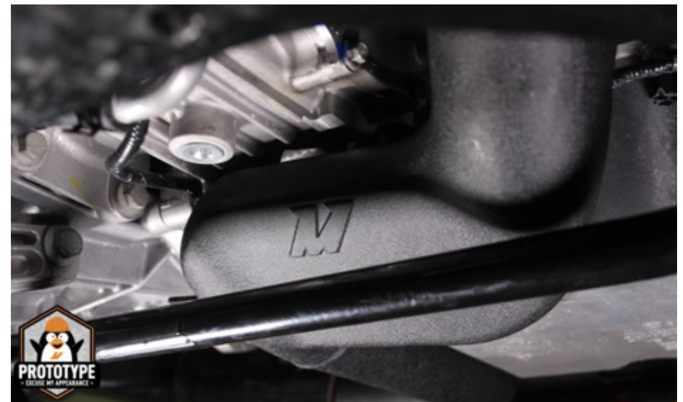
FIGURE 7: Image of the Mishimoto hot-side intercooler pipe installed.
