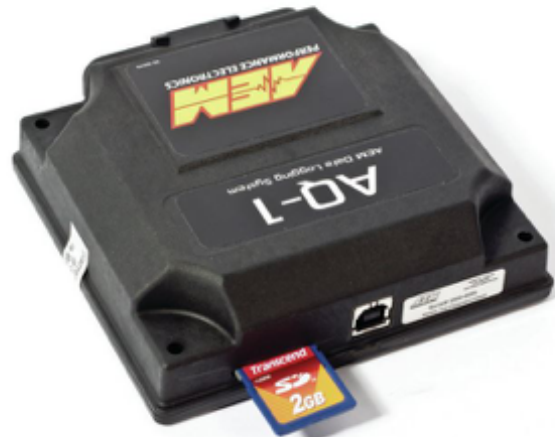
FIGURE 3: AEM AQ-1 Data Logging System.
