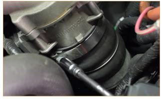
**03.** Remove the four bolts that secure the ducting to the front of the intercooler. [4x 10mm bolts]
