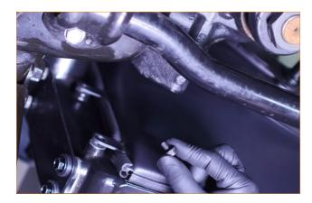
28. Locate the front ducting panels in your kit. Install the side panels by sliding them through the front grille. Then secure them with the four provided bolts. (4x 10mm bolts, 4x washers)
