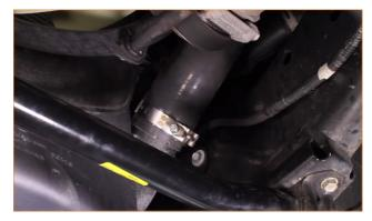
09. Loosen the clamp that secures the intercooler pipe to the driver side of the intercooler. (1x T-bolt clamp)
