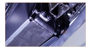
**30.** Install the two remaining bolts that secure the intercooler to the frame, and tighten all four bolts. (2x 13mm bolts)
