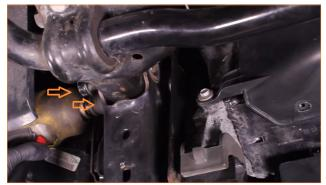
**08.** Loosen the clamp that secures the intercooler pipe to the passenger side of the intercooler. (1x 11mm T-bolt clamp)
