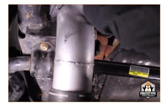
**22.** Route the cold-side intercooler pipe over the steering gear, and turn it while you feed it up toward the intake.
