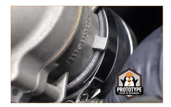
26. Slip two of the provided T-bolt clamps over the turbo end of the hot-side intercooler pipe. Install the pipe over the turbocharger outlet, but don't tighten the clamps yet. (2x T-bolt clamps)
