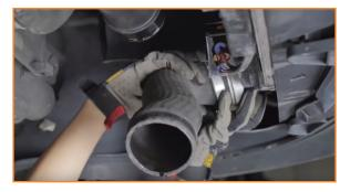
Loosen the clamp and release the clip from the hot-side coupler/hose, and then remove it. (1x worm gear clamp, 1x spring clip)
