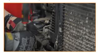
28. Separate the intercooler from the radiator. There is a bolt at each corner of the radiator. (4x T30 torx bolts)
