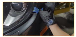
Remove the last two bolts securing the top of the bumper. (2x T25 torx)
