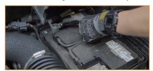
16. Unplug the yellow and red crash sensors as well as the headlight. Slide the red tab down and pull the connector out of the harness.
