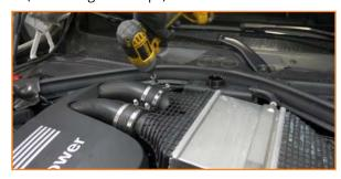
Separate the quick-disconnects from the intercooler. Lift the clip on each one to free the connections. Place something underneath to catch residual fluid from these connections. (3x spring clips)
