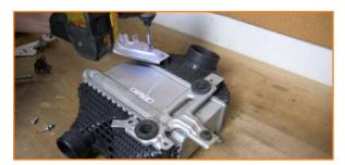
10. Transfer the brackets to the Mishimoto intercooler. Secure them using the provided hardware. (5x M5 3mm Allen bolts)
