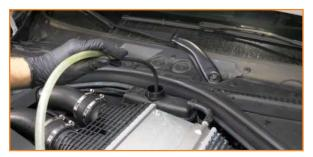
Disconnect the sensor on the side of the intercooler. Press the tab at the center of the connector to release the harness.
