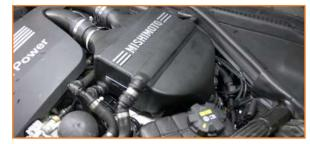
15. Reattach the quick-disconnects. (3x spring clips)
