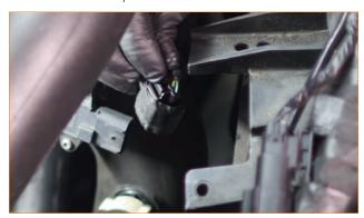
**06.** Disconnect the hose from the cold-side intercooler pipe. To release this connection, squeeze the tabs on the underside of the connector, and slide the locking clip away from the port.
