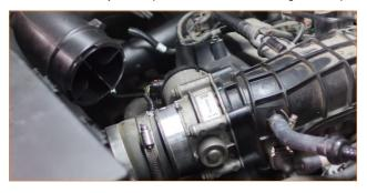
05. Disconnect the wiring harness from the sensor on the cold-side intercooler pipe. To release this connector, depress the black tab and pull the connector off the sensor.
