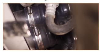
13. Separate the passenger-side intercooler pipe from the turbocharger outlet and the intercooler inlet. Release the peg in the middle of the pipe from the grommet that secures it to the engine, and then remove the pipe from the vehicle.
