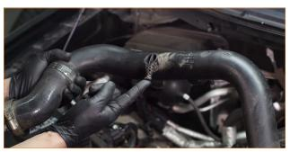
14. Separate the driver-side intercooler pipe from the turbocharger outlet. Lift up on the coolant expansion tank, and slip the intercooler pipe out from under it. There is a peg that secures this pipe to the engine directly under the coolant fitting on the expansion tank. Now separate the other side of the pipe from the intercooler and remove the pipe from the vehicle.
