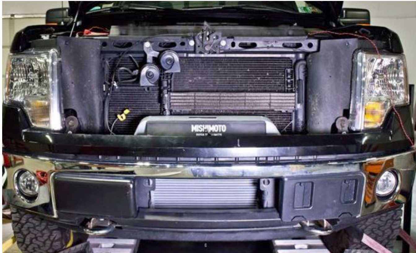
FIGURE 1: The Mishimoto intercooler features shrouding to direct ambient airflow through the core for maximum temperature reduction.
