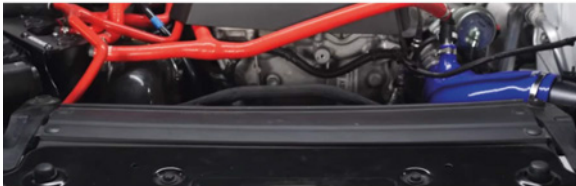
27. Remove the bolts that secure the AC condenser. Then, slide the condenser upward to free it from the tabs at the top. Lower the unit to give yourself some space to reach the intercooler. (2x 10mm bolts)
