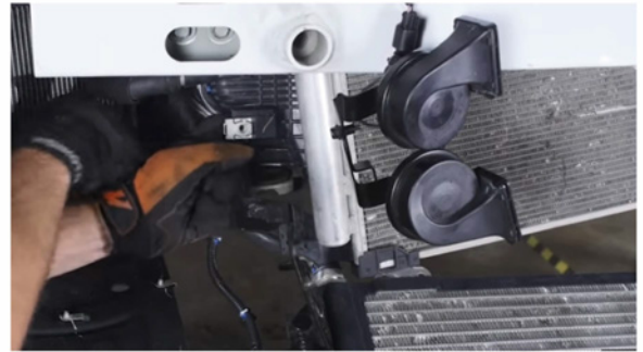
30. Remove the rubber shrouding on the driver side, in between the headlight and radiator. (1x pop-clip)
