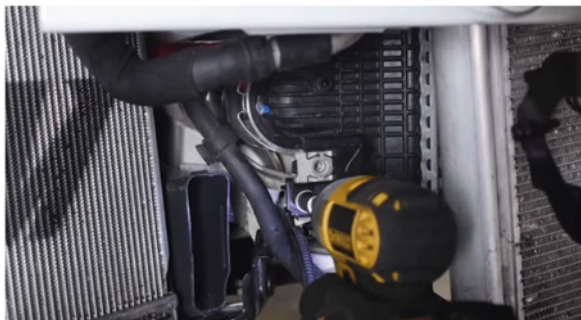
28. Remove the bolts that secure the lower section of the intercooler. (2x 10mm bolts)
