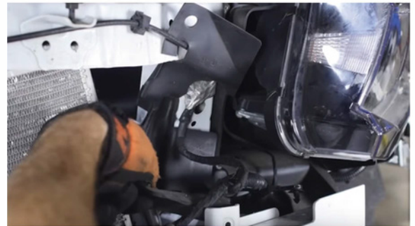
31. Lower the stock intercooler from the vehicle. 32. Install the Mishimoto intercooler by lifting it up into the same location as the stock component and letting it rest on the lower brackets. The AC condenser was removed for this image to give a better view of the step, but you can still install the part without removing the condenser.
