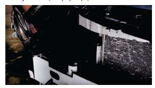
22. There are spring washers located around the stock radiator. Use a flathead screwdriver to wedge these free. (5x spring washers)
