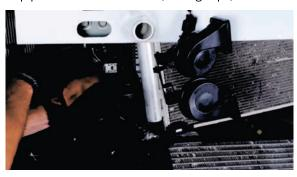
30. Remove the rubber shrouding on the driver side, in between the headlight and radiator. (1x pop-clip)
