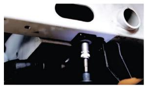
24. Separate the car horn from the front bumper. (1x 10mm bolt)
