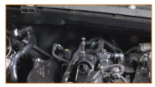
5. Disconnect the blow-off valve electrical harness. Lift the red tab and depress the black tab at the center to separate the connection.
