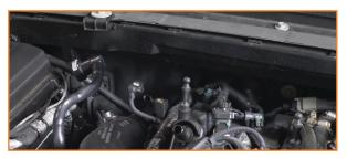
Loosen the clamps that hold the hoses on the intercooler pipe.
