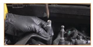
3. Release the breather attached to the heat shrouding. (2x pop-clips)
