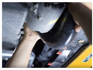
16. Tighten each clamp, making sure that the coupler is fully seated and the clamp isn't on the bead roll of either port. Reinstall the engine cover.
