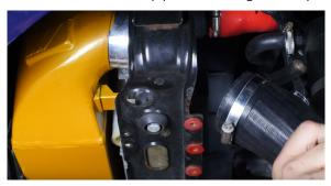
4. Slide a clamp over the shorter coupler in your kit and install it to the turbo. Leave the clamp loose for now. (1x worm gear clamp)
