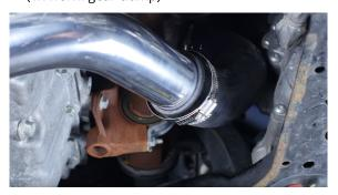
Align the pipe so it will fit in the crease between the transmission and oil pan without touching either. Rest the two brackets welded to the pipe on the studs you removed nuts from earlier. Secure the pipe with those original nuts. (1x 10mm nut, 1x 13mm nut)
