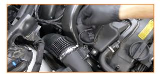
8. Remove the bolt that secures the remainder of the intake to the turbo. With the intake now free, remove it from the engine bay. (1x 10mm bolt)
