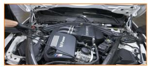
5. Lift the cover off the engine.
