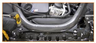
3. Remove the bolt that secures the primary expansion tank to the strut bar. (1x 10mm bolt)
