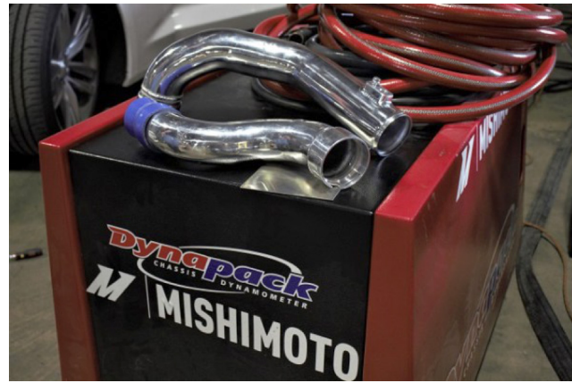
FIGURE 1: The Mishimoto intercooler piping is made from mandrel-bent aluminum piping to reduce bend angles and improve flow.
