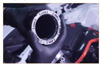
18. Remove the screw that secures the sensor to the cold-side pipe. Then remove the sensor by pulling it directly outward. Transfer the sensor to the Mishimoto cold-side pipe, and secure it with the provided bolt. Do not reuse the original screw on the Mishimoto cold-side pipe. (1x T20 screw, 1x 10mm bolt)
