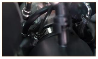
03. Disconnect the CCV hose from the intake by sliding the locking tab over and pulling the hose off the port.
