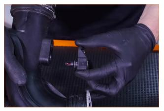
19. Inside the quick-disconnect fitting on each pipe, there is a rubber seal. Transfer the seals from the stock pipes to the Mishimoto pipes, taking care not to reverse the direction of the seals.
