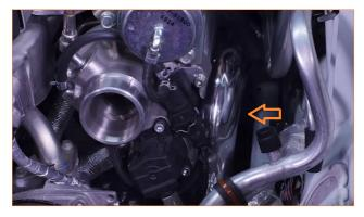
27. Lubricate the transition coupler, and install the wider end over the lower section of the hot-side pipe. Then slip the wider clamp over the coupler, followed by the smaller clamp. Lubricate the upper section of the hot-side pipe and lower it into place. Slip it into the coupler, and turn the pipe until the two-bolt flange aligns with the turbo outlet flange. (2x T-bolt clamps)
