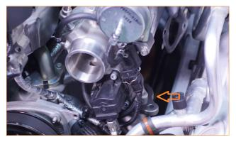
10. Disconnect the cold-side pipe from the throttle body. There is a gray lock-ring that secures this connection. To separate the pipe, turn the gray ring counterclockwise, and pull the pipe off the throttle body.
