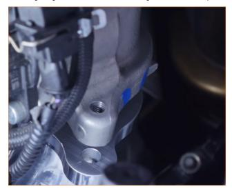
**28.** Reinstall the turbo charger gasket between the hot-side pipe and the turbocharger outlet. Then install the two original bolts to secure the pipe and tighten them completely. (2x 13mm bolt)
