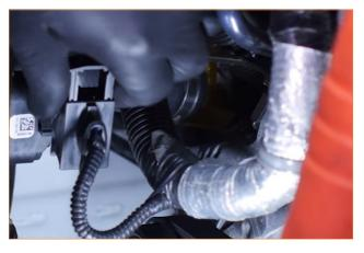
12. Reach down through the engine bay on the passenger side, and use a pick to lift the circlip on the cold-side pipe until it locks into the detent, as shown here. This detent will hold the circlip in the unlocked position.
