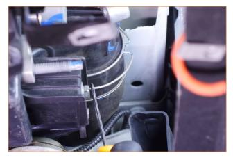
16. Remove the hot-side pipe from the vehicle. The pipe can be separated into two pieces by loosening the worm gear clamp. To remove it in one piece, slide it back toward the firewall, and feed the intercooler connection past the turbo first.
