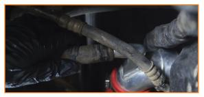
14. Use the two provided zip ties to connect the lower radiator hose to the lower support frame. Cut the excess zip tie once they are fully tightened.
