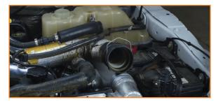
3. Pull the clip from the other end of the radiator hose and separate the connection. (1x spring clip)
