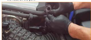
02. Compress the clamp that secures the sound generator tube to the intake hose and separate the tube from the hose.
