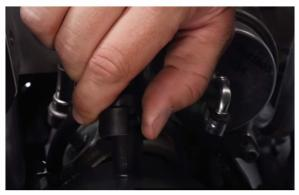
Loosen the two worm gear clamps securing the induction hose to the airbox and turbo. (2x worm gear clamps)
