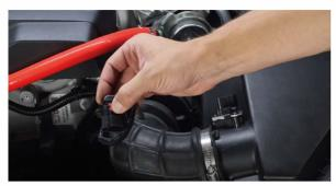
2. Separate the crankcase ventilation (CCV) hose from the induction hose. If you're working on a 2013+ Cadillac ATS or 2016+ Camaro 2.0T, then you will lift the small black tab on the connector and slide it over before pulling the hose off the port. For 2017+ models, there is a non-removable clip. Use the provided pick tools to slide under the connector and depress the two tabs inside.
