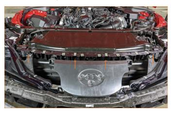
**08.** Remove the top metal radiator cover. Lift out of place once bolts are removed. (13x 13mm bolts)
