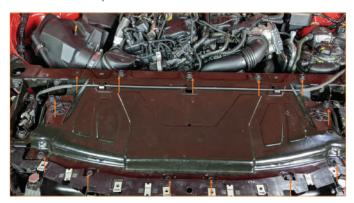
34. Reinstall the upper bumper bolt bracket. (4x 10mm bolts)
