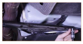
**02.** Remove the two nuts from the flange that attaches to the downpipe. (2x 15mm nuts)
