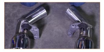
14. Slide a clamp over the driver-side exhaust and connect the tip assembly. Then lift the exhaust system and tip assembly upward, and slide the bracket over the bolts behind the bumper. The exhaust tip should fit into the available slot on the bumper. Repeat this process for the passenger-side tip assembly. (2x exhaust band clamps)
