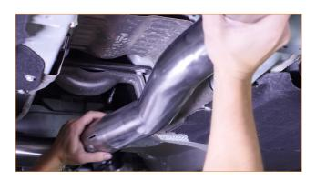
09. Slide a clamp over the mid pipe. Then install the rear pipe, which has a hanger welded to it, over the open end of the mid pipe. (1x exhaust band clamp)
