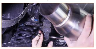
13. Organize the two exhaust tips in your kit so that they are positioned as though they were attached to the vehicle, each one with their hangers facing upward. Slide the driver-side and passenger-side brackets over the hangers on each tip assembly. The brackets are labeled, Rear Face Right Hand for the passenger side and Rear Face Left Hand for the driver side. Lubricate the rubber grommet on the bracket to help with this step.
