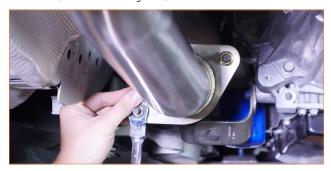
08. Slide a clamp over the front pipe you just installed. Then install the mid pipe over the open end on the front pipe. (1x exhaust band clamp)
