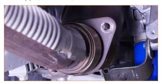
03. Use an exhaust hanger removal tool to pull the front bushing brackets from the exhaust hangers. Swing the bushing brackets to the side and out of the way once you've separated them. Repeat the process for the rear hangers.
