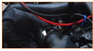
11. Slide the intake manifold forward to reach the clamp on the PCV hose.
