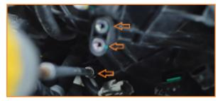
6. Remove the bolts that secure the coil pack wire cover to the valve cover. (2x 10mm bolts)
