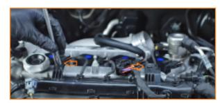
Remove the bolt that secures the vacuum line to the intake manifold. (1x 10mm bolt)
