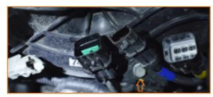
Remove the bolt on the bracket that holds the coolant line to the intake manifold. (5x 10mm bolts)
