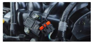
4. Remove the bolt on the bracket that holds the bottom sensors. (1x 10mm bolt)
