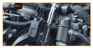
8. Separate the positive terminal on the alternator. (1x 12/13mm nut)
