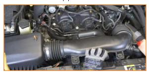
10. Remove the bolts that secure the vacuum pump to the bracket. Do not remove the pump.
