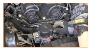
11. Lift the vacuum pump slightly so that you have enough room to slide the catch can brack under the pump. Align the holes in the bracket with the pump's grommets. With the bracket set, secure the bump using the original hardware. (2x 10mm bolts)
