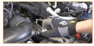
Remove the bolts that secure the intake brackets. (2x 10mm bolts)
