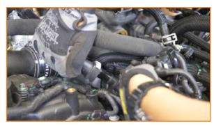
Separate the intake air temp sensor wiring from the intake pipe. Next, disconnect the sensor electrical harness from the intake.
