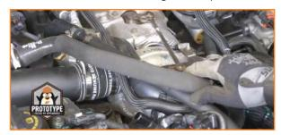
15. Connect the Mishimoto outlet hose to the PCV heater and push the yellow tab to secure the connection. The fitting should click twice.
