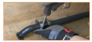
14. Route the hose with the rubber elbow under the bypass valve pipe and connect it to the valve cover. Route the other end under the turbocharger muffler and connect it to the IN port on the catch can. (1x worm gear clamp)
