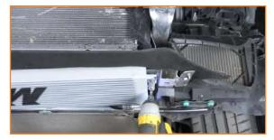
15. Remove the bolts on the lower part of the clam shell. (2x T25 plastic screws)
