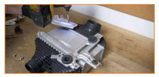
10. Transfer the brackets to the Mishimoto intercooler. Secure them using the provided hardware. (5x M5 3mm Allen bolts)
