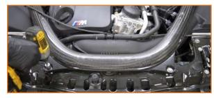
Remove the bolt that secures the primary expansion tank to the strut bar. (1x 10mm bolt)
