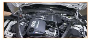
Lift the cover off the engine.
