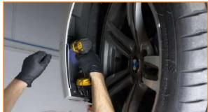
4. Pull back the wheel well liner to gain access behind it. Remove the bolts that secure the bumper to the edge of the fender.
