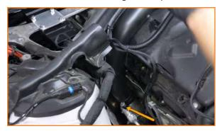
14. Attach a silicone coupler to the front intercooler pipe. Then set the front pipe and slide the coupler onto the intercooler.(1x E11 torx bolt, 2x worm gear clamps)
