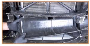
12. Remove the bolts that secure the cross brace and slide it out from behind the upper ducting. (6x T45 torx)
