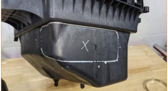
Reassemble the air intake. Remove the stock fresh air duct and seal the port with provided rubber plug. Note that the plug must be sealed with RTV, silicone caulk or butyl tape if intend to use for water fording. Reinstall the air intake back on the vehicle.
