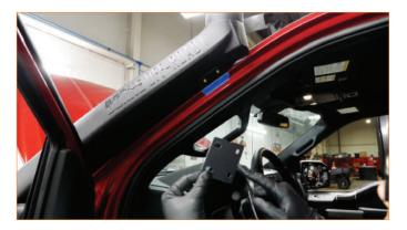
Secure the A-pillar bracket to the A-pillar rivet nuts with provided 2x M4 button head flange bolts. Remove the two long bolts securing the snorkel body to the fender tube, apply Loctite on the tip of the bolts then re-install them. Adjust and tighten all snorkel fasteners.
