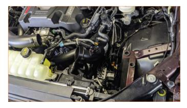
**02.** Release all harness clips from wheel well liner, push them toward the firewall and secure with provided zip ties. Area indicated by the arrow must be free of wire harnesses. Release the thick main harness wire loom that runs along the fender frame, lift it up and secure with provided tree clip zip tie.
