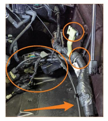
**03.** Remove the fender flare. Remove the 5x screws securing the flare to the wheel well liner, then pull the flare away from the fender to release the clips. Disconnect the marker harness before completely removing the flare.
