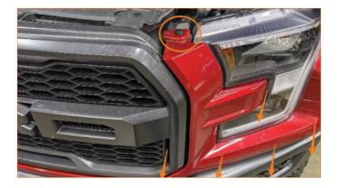
**06.** Remove the headlight bracket. Remove 6x fasteners from the front and side of the bracket, then release the marker harness from the bracket. Pinch the clip circled just above the bolt to release it and remove the bracket.
