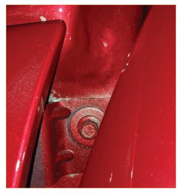
> Lift the corner of the cowl to expose the bolt underneath.
