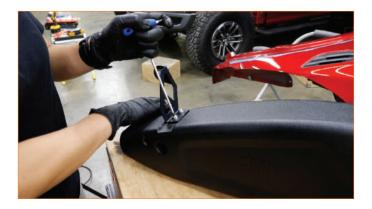
13. Install the provided rubber grommet on the fender frame as shown, then install the rubber duct onto the stock intake adapter port or the Mishimoto intake side inlet port. Install the Borne Off-road snorkel fender tube assembly by engaging the peg with the grommet and connect the fender tube port with the rubber duct. Note that the rubber duct connections should be secured with zip ties if intend to use for water fording.
