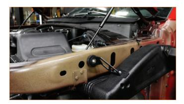
14. Reverse steps 5-9 and reinstall the headlight, fender headlight bracket and trim piece. Check to make sure the drilled holes on the fender line up with the threaded holes on the Borne Off-road snorkel fender tube.
