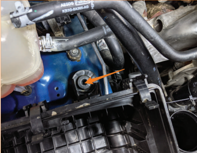
03. Remove fender vent cover by pulling outward.
