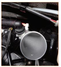
8. Reinstall the air intake tube. (1x worm gear clamp, 1x spring clamp)
