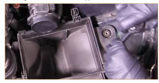
05. Remove the rubber airbox bushing from the frame rail by pulling it up off the studs.
