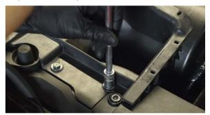
Loosen the bolts that secure the airbox. It will be difficult to completely remove the lower bolts at the moment, so for now just loosen them all the way. They will come out when you remove the airbox.
