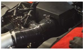
28. Install the jet valve to the intake tube. Attach both hoses and secure them with the available clamps. (1x worm gear clamp, 2x spring clamps)
