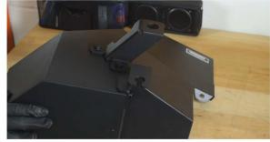
20. Transfer both bushings as well as the grommet and the air duct's rubber liner onto the Mishimoto airbox.
