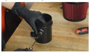
25. Insert the MAF housing to the airbox's lid. Make sure the edge of the hole on the lid is properly seated on the rubber gasket. Then install the housing to the filter. (1x worm gear clamp)
