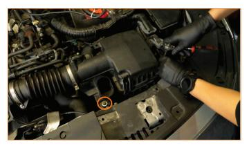
**5.** Remove airbox from the engine bay. Make sure the bottom rubber grommet comes out with the airbox.
