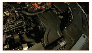
**11.** Install the silicone hose and 2x worm gear clamps, then tighten down the airbox with the provided hardware. (2x 10mm bolts and washers)
