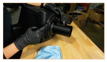
**10.** Install the airbox assembly, push down to engage the bottom grommet with the metal peg in the engine bay.
