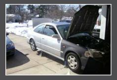
Remove radiator cap. Crawl under the car and open petcock to drain the coolant from the system. Once it is slowly dripping, you can squeeze the lower (and possibly the upper) hoses to get more of the coolant out. If you plan on re-using the coolant, have a clean drain pan underneath it.
